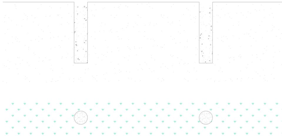
3. Fill the hole with post mix (use manufacturer's instructions). Adjust post into position and support until post mix sets.
